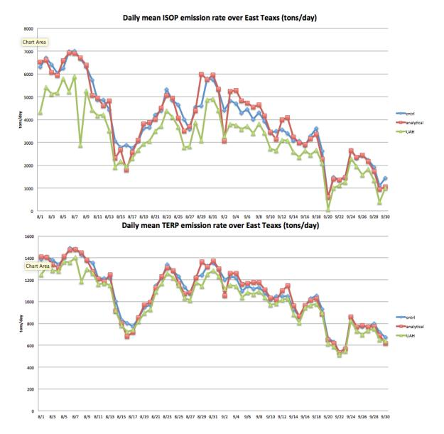
Figure 5. Comparison of the daily variation of isoprene (ISOP, top) and monoterpene (TERP, bottom) emission rate (tons/day) over East Texas during August and September 2013 by MEGAN using different PAR inputs.
